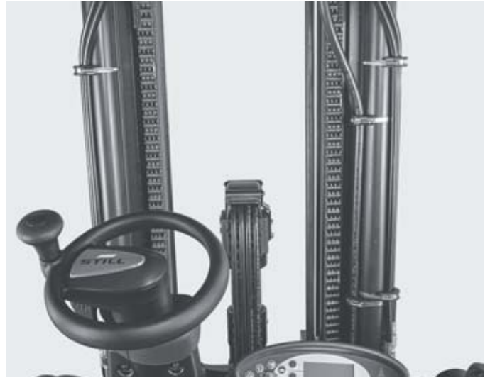
Free view with triplex mast
