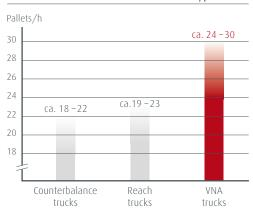
Assuming a racking beam height of 6 metres and an average work efficiency, counterbalance trucks can move around 18 – 22 pallets per hour. Reach trucks can handle around 19 – 23 pallets per hour (but only 16 in Drive-In racking and only 13 in double deep). By contrast, VNA trucks achieve by far the highest performance handling 24 – 30 pallets per hour.
