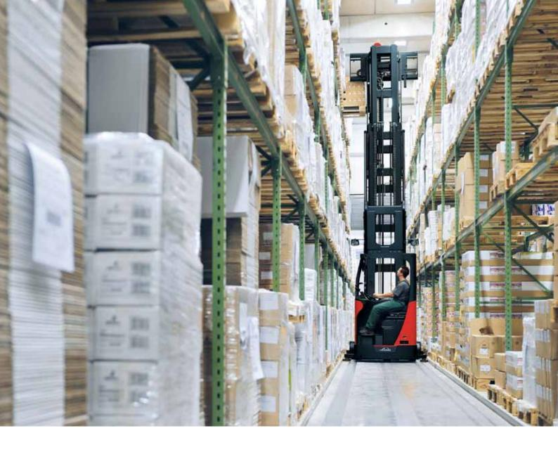
**Safety.** VNA provides the maximum security in pallet handling resulting in considerably less product and racking damage. Thus VNA solutions are ideal, if high value goods are handled and damage costs are causing problems. By being on the same level when storing pallets with a guided truck, damages can be significantly reduced.
