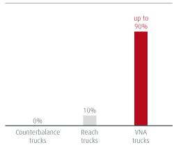
Depending on the truck type, product and rack damage differ. The percentages shown are the maximum cost savings that result from replacing different truck types. By using a VNA truck, the costs resulting from damages can be reduced by up to 90%.
