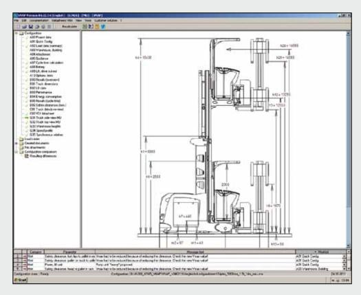
After collecting all relevant data, the final truck specification is displayed by the software. The software also generates the aisle dimensions, the achievable performance data, the energy consumption, etc. on the spot.
