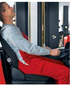
**Seat:** Hydraulically damped seat with lumbar support. Flexible and adjustable for visibility when placing or retrieving pallets. Available with a heater option.
