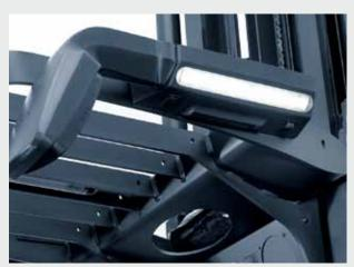
**LED:** The bright LED working lights guarantee good visibility into the racks. Powerful ventilation fans are adjustable in two steps
