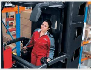
**Mirror module:** Best visibility onto guide rollers and over truck rear
