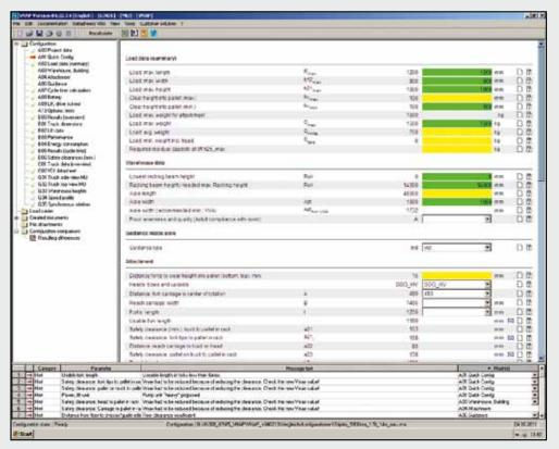
In order to create the perfectly adapted truck, all relevant warehouse and application data needs to be collected. Starting with the load dimensions, the racking details, type of guidance, battery size etc. all information is put into the software tool.
