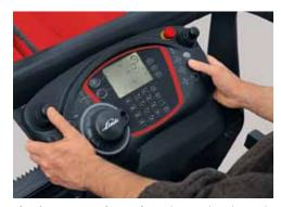
**The front Control Panel** can be easily adjusted for height, distance and tilt to suit each operator. The display shows all relevant truck operating data
