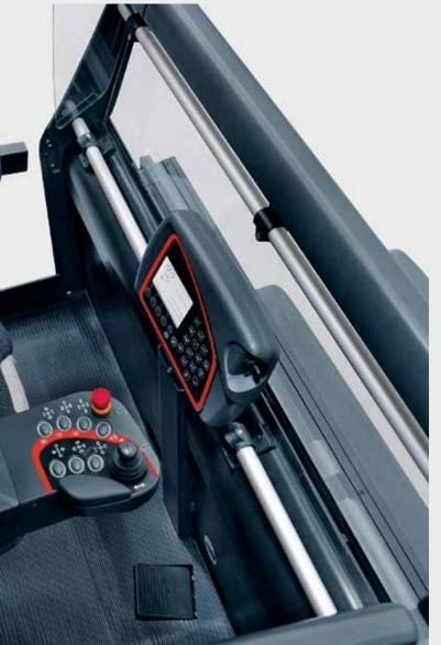
**Flexible mounting and storage system:** The mounting system allows individual attachments such as monitors and scanners, and Linde attachments such as storage utilities, clipboard, etc. to be integrated into the truck cabin
