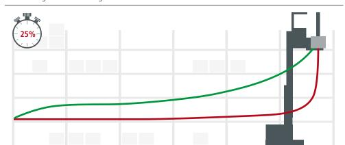
Optimised operation with storage navigation provides a time saving of up to 25%. The green line shows the shortest time using the fastest route and with as little energy used as possible.
